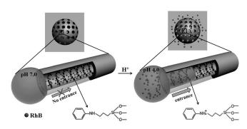
**Scheme 1.** The release process of the pH-responsive free-blockage controlled release system based on MSNs. This system can release Rhodamine B in acidic conditions.
