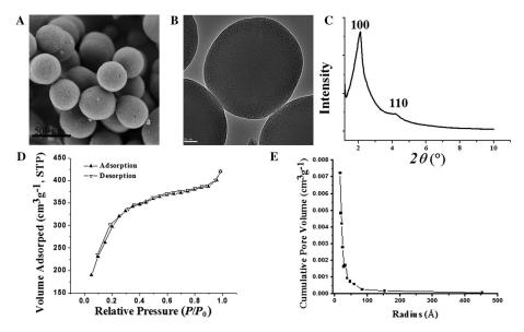
Figure 2. A) SEM image: the average diameter of MS-Ph (1:20) was around 300 nm. B) TEM image: the mesoporous channel could be clearly observed by transmission electron microscopy; scale bar: 50 nm. C) XRD results: a lattice spacing of approximately 4.2 nm was observed. D) N<sub>2</sub> sorption isotherm of MS-Ph (1:20). E) The distribution of pore size of MS-Ph (1:20).
