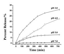
**Figure 3.** pH dependence of the release profiles of RhB-loaded MS-Ph (1:20). The release gradually sped up as the pH value was reduced.
