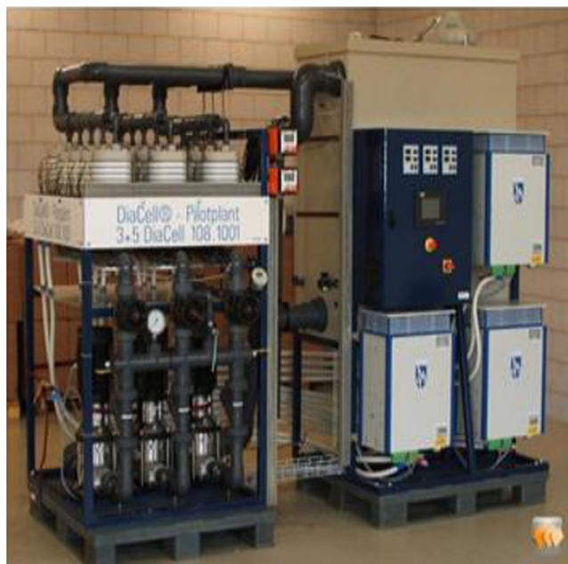
Fig. 4 EAOP pilot plant for the treatment of landfill leachate in Marelo (Cantabria, Spain) (Anglada et al. 2009, 2010, 2011; Urtiaga et al. 2009)
