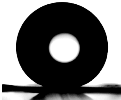
Fig. 3. Shape of water droplet on the dried PANI modified PAA membrane surface after being immersed in 1 \text{ mol L}^{-1} HCl solution at 60^\circ \text{C} for 6 h.
