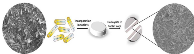
Figure 8. SEM images showing uncompressed drug loaded nanotubes (left) and bound nanotubes (right) compressed in the tablet core. Adapted from ref. 28 with permission from Elsevier.
