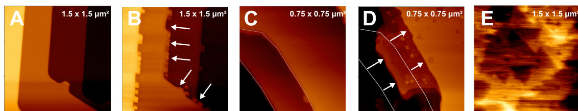
Figure 4. In-situ AFM topographies indicate preferential dissolution of 10\bar{1} step edge surfaces on a (0001) surface (marked by arrows) upon decrease of the pH values from (A/B) pH 8–6 and (C/D) pH 8 to pH 3. Panel E shows an ex-situ topography after immersion into a pH 3 solution, indicating stabilization by formation of triangles with step edges of (10\bar{1}) orientation on (0001) surfaces (c.f., text for details).
