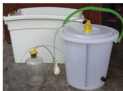
The experiment to verify the volume of gas produced from the reaction of \text{NaHCO}_3 and \text{HCl} that is used in creating a useful thing in the second lesson.
