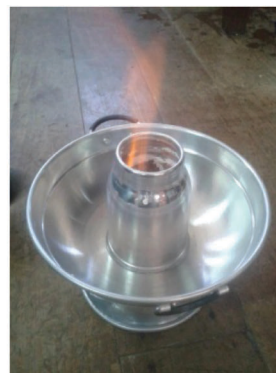
Various applications by using the fuel jelly produced from the reaction of \text{Ca}(\text{OH})_2 , \text{CH}_3\text{COOH} and \text{C}_2\text{H}_5\text{OH} .
