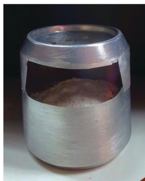
Various applications by using the fuel jelly produced from the reaction of \text{Ca}(\text{OH})_2 , \text{CH}_3\text{COOH} and \text{C}_2\text{H}_5\text{OH} .
