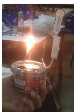
Some useful things acquired from the reaction of \text{CaC}_2 and \text{H}_2\text{O} .
