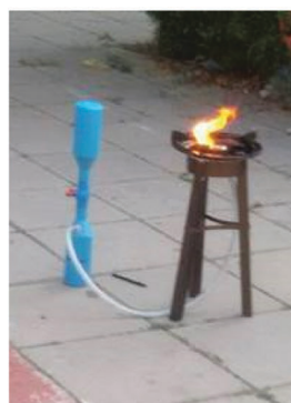
Some useful things acquired from the reaction of \text{CaC}_2 and \text{H}_2\text{O} .
