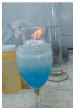
Various applications by using the fuel jelly produced from the reaction of \text{Ca}(\text{OH})_2 , \text{CH}_3\text{COOH} and \text{C}_2\text{H}_5\text{OH} .
