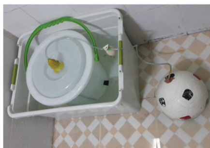
The experiment to verify the volume of gas produced from the reaction of \text{NaHCO}_3 and \text{HCl} that is used in creating a useful thing in the second lesson.
