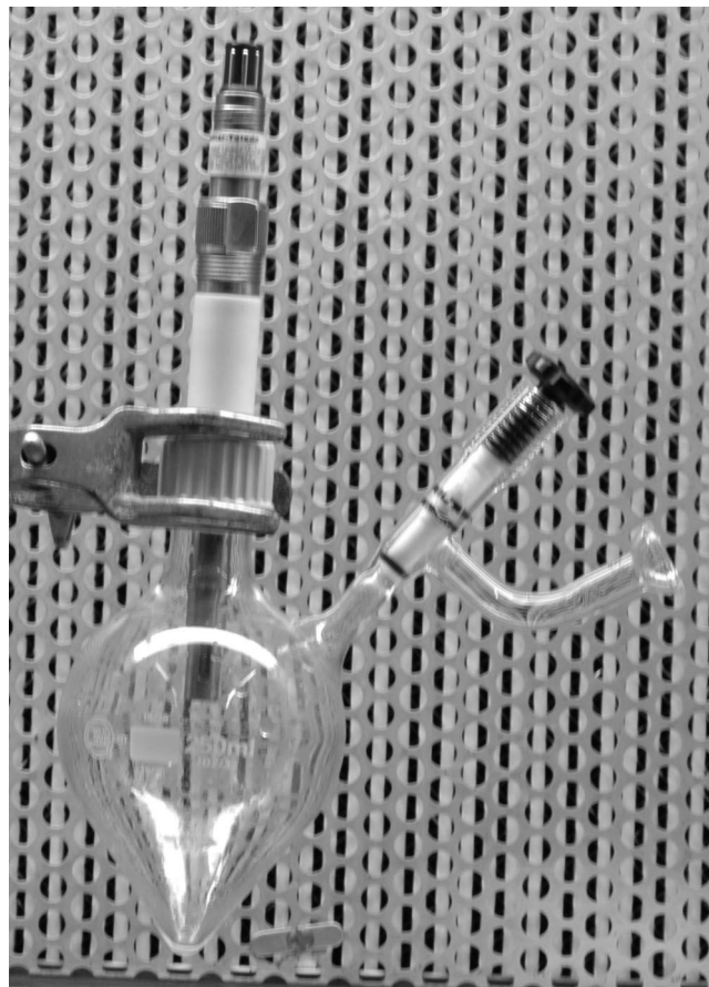
Figure 1. Conductivity vessel: Mettler Toledo 7001/120 VP 3.1 B probe sealed in pear shape flask via PTFE sleeve.
