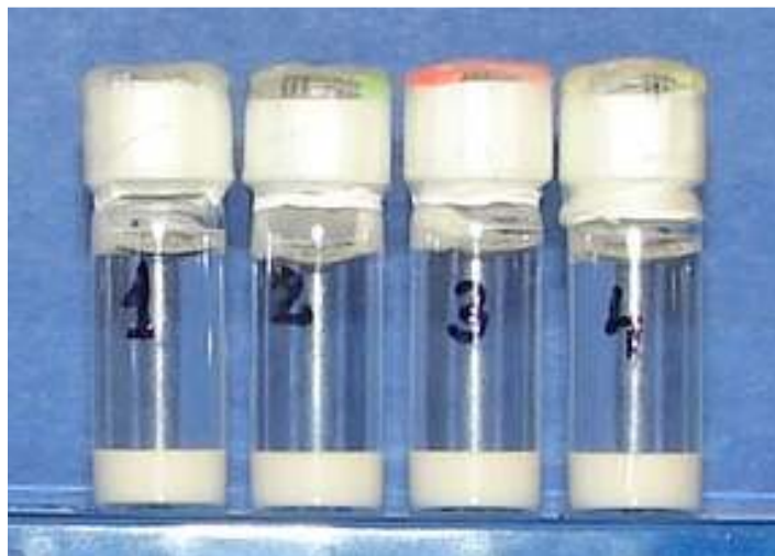
Fig. I.1. Samples with sedimented particles in aqueous surfactant solution.
