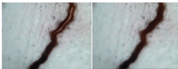
Fig. 3 Microscope photos of self-healing coating films with urea–formaldehyde microcapsules immediately after crack formation (left) and after 90 s (right). 28
