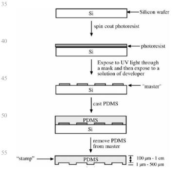
**Fig. 1** Diagram illustrating the fabrication of a PDMS stamp. (Reprinted with permission from ref. 26. Copyright 1999 Elsevier.)
