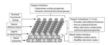
**Fig. 3** Diagram showing the binding of the thiol group in alkanethiols to a metal substrate to form crystalline self-assembled monolayers presenting a terminal functional group. (Reprinted with permission from ref. 27. Copyright 2005 American Chemical Society.)
