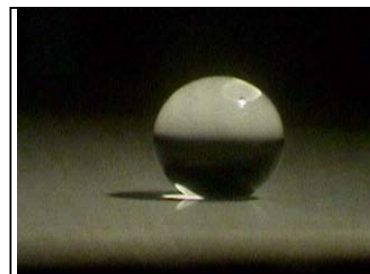
Fig.5. A droplet of 1M HCl on a top of fluorinated alumina membrane. The contact angle, \theta > 150^\circ , does no change with time.
