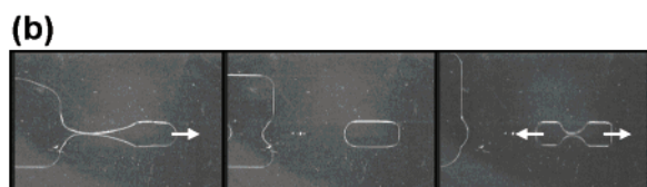
A single droplet is created from a reservoir and split into 2 droplets.
