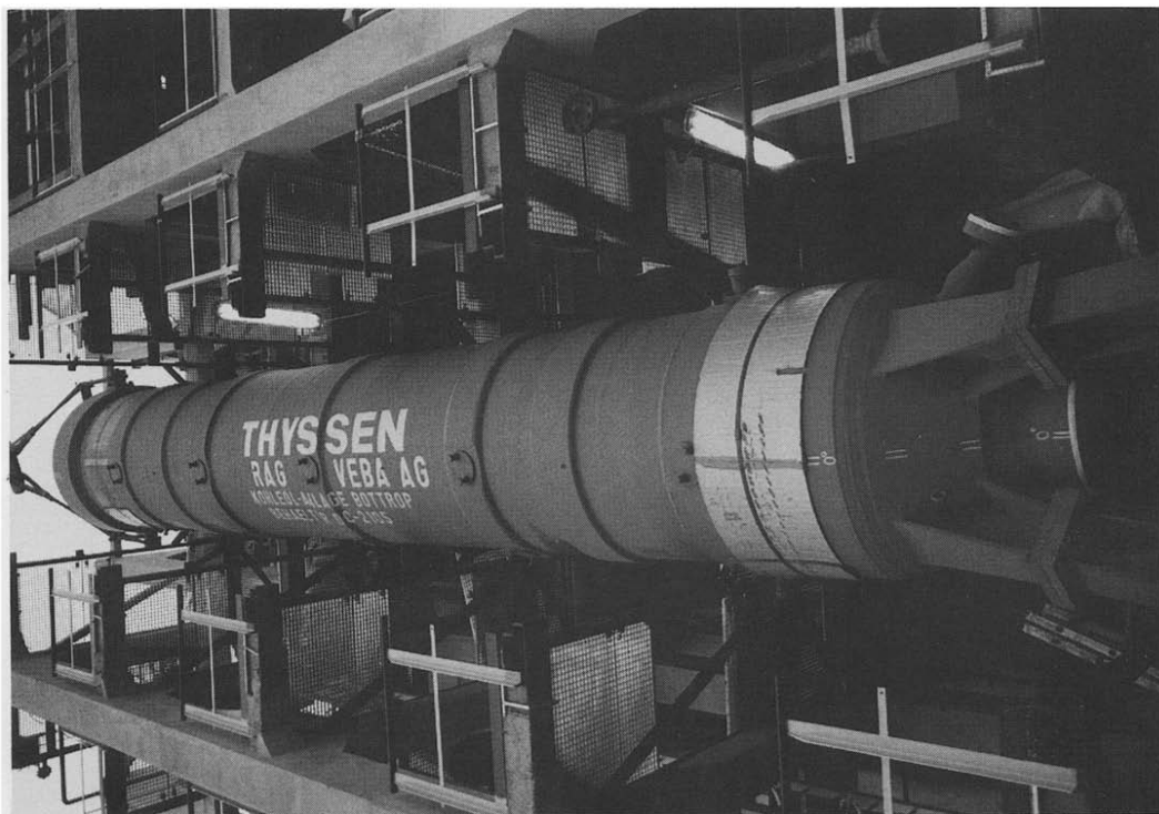
Fig. 13. Large volume reactor of the Demonstration Plant Bottrop.
