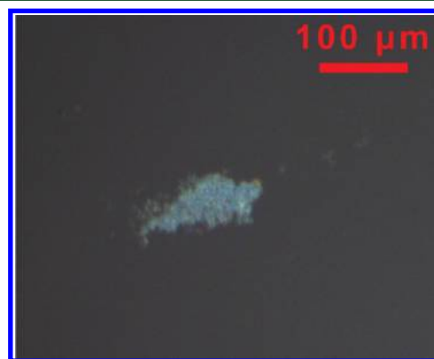
Figure 4. Photomicrograph of initial mesophase observed during cracking Athabasca bitumen under hydrogen at 4.8 MPa and 440 °C with agitation at 140 rpm as an aggregated domain.
