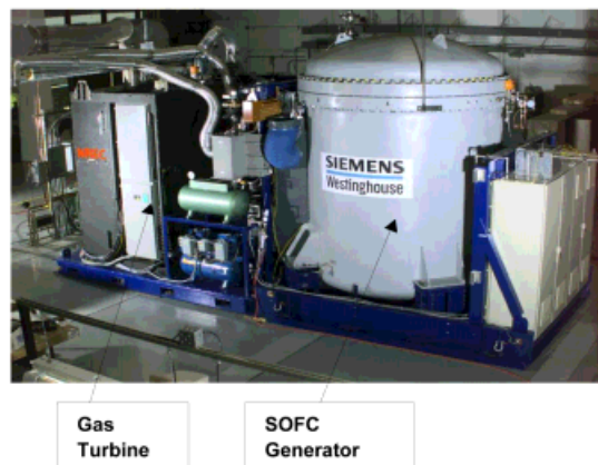
Fig. 27 Combination of a pressurised SOFC with a micro-gas turbine. Concept of Siemens-Westinghouse.
